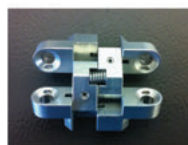
SH105-A-Open Limited travel hinge Adjustable, Springs Open
