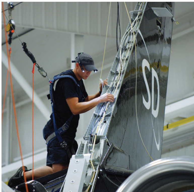
Preparing for the SD Plane Simple™ Ku-band tail mount antenna install
