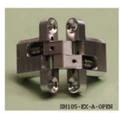
SH105-EX-A-Open Limited travel, Adjustable hinge, Compression springs for added force
